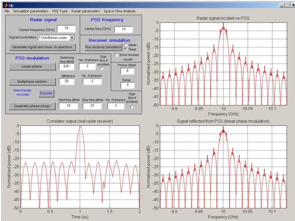
Figure 1 Layout of PSSim GUI (simulation of 13 bit Barker coded pulse radar)
