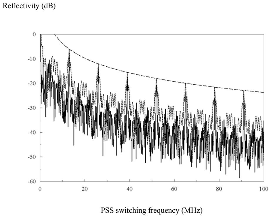
Figure 4 Performance of PSS against radar with uncoded (\_\_\_), 13 bit coded (...) and 51 bit (\_\_\_) coded pulses
