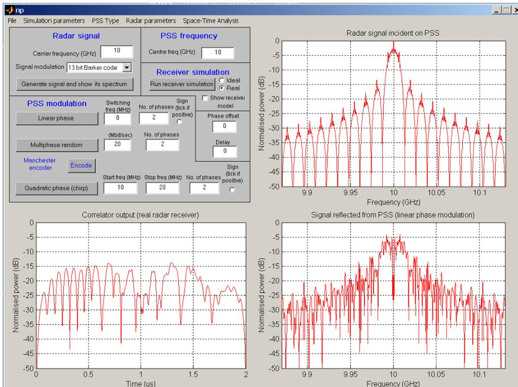
Figure 2 PSS switched at 8 MHz and operating against 13 bit Barker coded pulse radar
