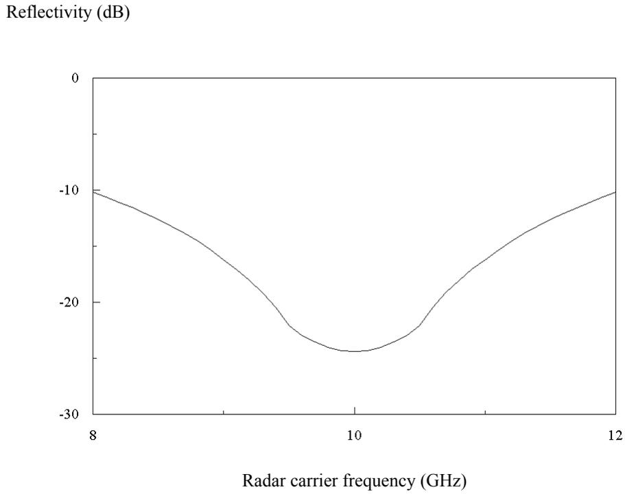
Figure 3 Effective PSS reflectivity as measured by pulse compression radar (51 bit code, 30 MHz switching frequency, 10 GHz PSS centre frequency)
