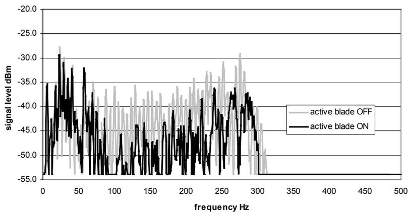
Figure 3 Measured reflected Doppler spectrum from PSS coated wind turbine
