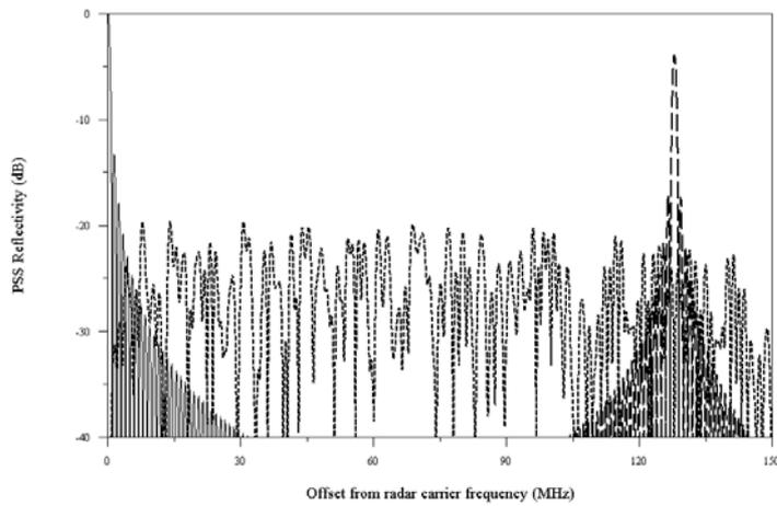
Figure 1 Predicted spectra of incident radar signal, PSS reflected signal with regular square wave switching and PSS reflected signal using 256 bit code
