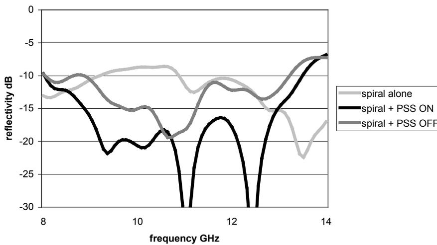
Figure 2 Measured reflectivity response of cavity-backed spiral antenna with PSS boundary
