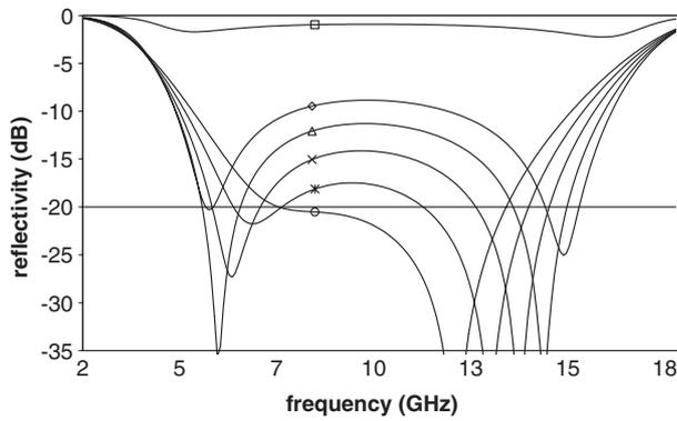
**Figure 4.** Predicted reflectivity response of a single-layer absorber with a series equivalent impedance described by  $Z_s = R_s + j\omega L_s + 1/j\omega C_s$ , with  $L_s = 3.4$  nH and  $C_s = 9.1$  fF and  $R_s$ :  $\square = 20 \Omega$ ,  $\diamond = 180 \Omega$ ,  $\triangle = 220 \Omega$ ,  $\times = 260 \Omega$ ,  $*$  =  $300 \Omega$ ,  $\circ = 340 \Omega$ .
