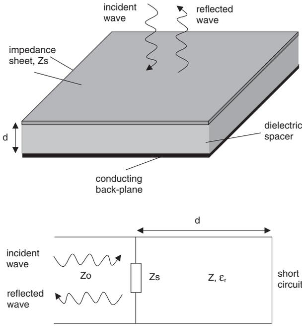
**Figure 1.** A single-layer planar absorber (top) and transmission line equivalent circuit (bottom).
