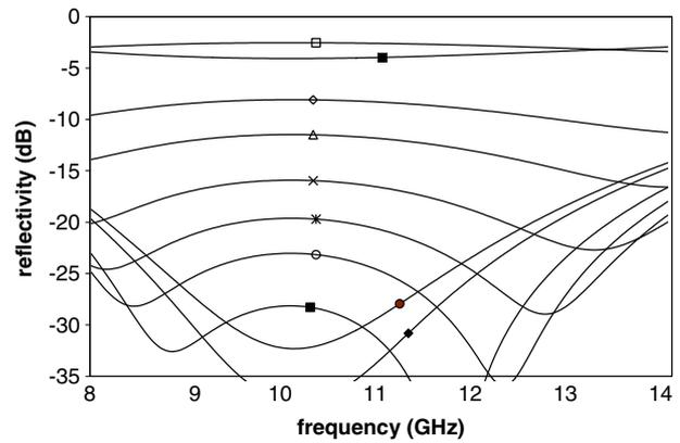
**Figure 8.** Predicted reflectivity characteristics of the single-layer active absorber using the model in figure 7 with  $C = 4.9$  fF,  $L = 4.7$  nH,  $R$ ,  $\square = 50$   $\Omega$ ,  $\diamond = 150$   $\Omega$ ,  $\triangle = 200$   $\Omega$ ,  $\times = 250$   $\Omega$ ,  $*$  = 280  $\Omega$ ,  $\circ = 300$   $\Omega$ ,  $\blacksquare = 320$   $\Omega$ ,  $\blacklozenge = 350$   $\Omega$ ,  $\bullet = 360$   $\Omega$ ,  $\blacksquare = 1500$   $\Omega$ .
