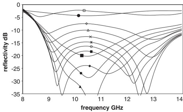
**Figure 6.** Measured absorber reflectivity as a function of diode bias current.  $\square = 0.0$  mA,  $\diamond = 0.025$  mA,  $\triangle = 0.05$  mA,  $\times = 0.06$  mA,  $*$  = 0.07 mA,  $\circ = 0.075$  mA,  $\blacksquare = 0.085$  mA,  $\blacktriangle = 0.1$  mA,  $\bullet = 0.11$  mA,  $\blacksquare = 0.13$  mA,  $\bullet = 1.0$  mA.
