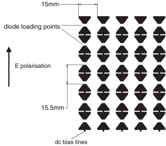
**Figure 5.** Details of the linearly polarized active FSS topology.
