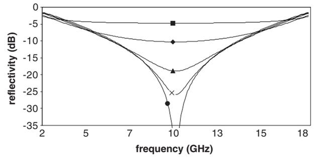
**Figure 3.** Variation in reflectivity with sheet resistance for a 10 GHz Salisbury screen. Sheet resistance values ( $\Omega/\square$ ): ■ = 50 or 2838, ◆ = 100 or 1419, ▲ = 300 or 473, × = 340 or 417, ● = 377. Note that the high and low values of sheet resistance are related by the formula  $Z_{high}Z_{low} = Z_0^2$  and therefore give identical reflectivity curves.
