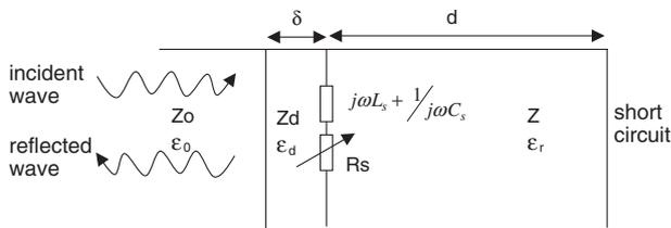
**Figure 7.** Transmission line equivalent circuit of the experimental active absorber with outer dielectric skin of thickness  $\delta$ .
