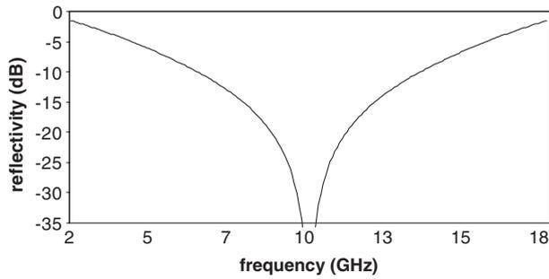
**Figure 2.** Reflectivity characteristics of a Salisbury screen designed for operation at 10 GHz.
